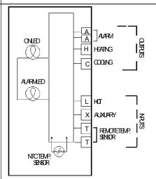
Model Number: TE401140; 120 vac Description: Electric heat or cool SPDT
